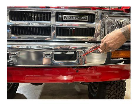
2. Install new supplied hardware from behind the behind the bumper into the light bar.
